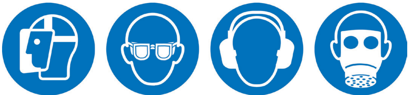
Figure 3: Current ISO symbols for “Wear Face Shield,” “Wear Eye Protection,” “Wear Ear Protection,” and “Wear Respiratory Protection”.
